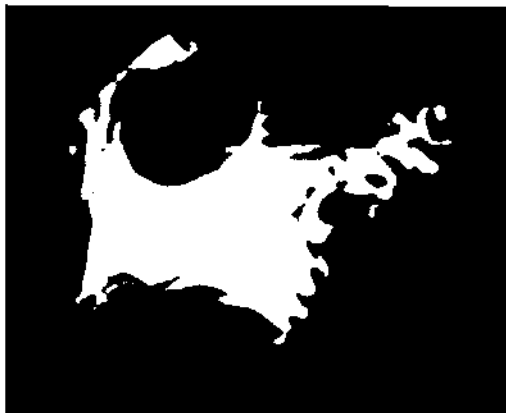
Figure 11. NO–H 2 /Rh(111); development of the spiral and the region of reduced work function at 456 K with p(\text{NO}) = 1 \times 10^{-6} mbar and \text{H}_2/\text{NO} = 6.5 (from reference [91]). The diameter of the image is about 600 \mu\text{m} .
